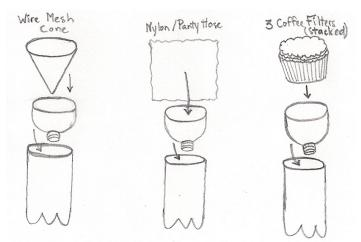
The nylon pieces should be relatively loosely fastened using tape so that they reach the bottom of the bottle top funnel. Refer to the above-right for an illustration of this. Make sure that each group has their separate filters in the order of wire mesh, nylon and then coffee filters.
