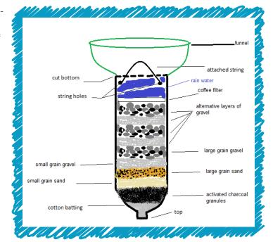
The untreated water will work through the layers of sediment to wick away the impurities in the water. The cotton batting catches particulates from the sediment and acts as a final buffer.
